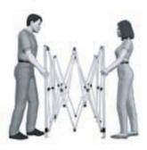
Remove assembly from portable, wheeled storage bag. Grab corner legs in each hand. Lift frame slightly off ground. Stepping backwards, pull frame apart until your arms are fully extended.
