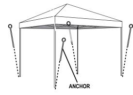
For temporary anchoring of canopy on grass, dirt or packed soil, insert temporary spike anchors through corner feet.
